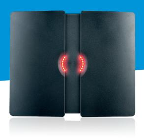
Several communication interfaces are available such as RS232 (default, standard included), RS422, RS485, HID Interface Board (HIB) and TCP/IP. Also open industry-standards protocols such as Wiegand are supported. Customer specific protocols can be implemented on request.
